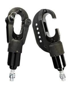
The new light weight 15-ton Y46LWBH Latch Head and Y46LWSBH C-Head remote operated crimping tools have been redesigned with new forged heads that offer a weight reduction of more than 10%. Additionally, these tools continue to accept all standard BURNDY<sup>®</sup> "P" & "U" style crimping dies (w/PUADP-1 adapter).
